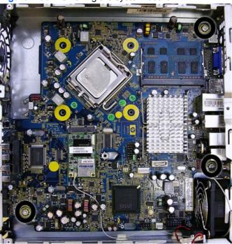
Figure 7-36 Removing the system board
